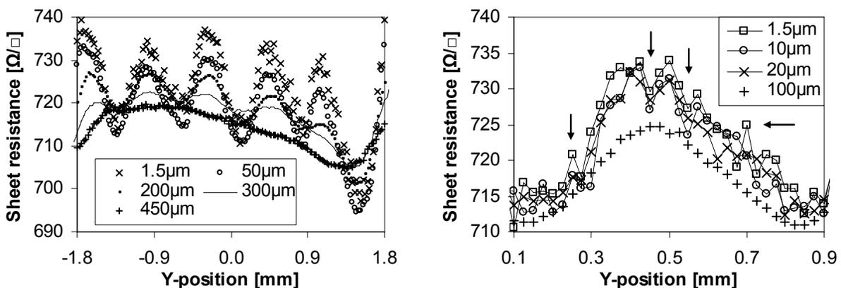
Figure 5: Selected probe pitch and line segment of the 5 mm line scan in figure 3. A line segment was chosen to represent the two main periodic variations of 3.65 mm (left) and  $\sim 750 \mu\text{m}$  (right).
