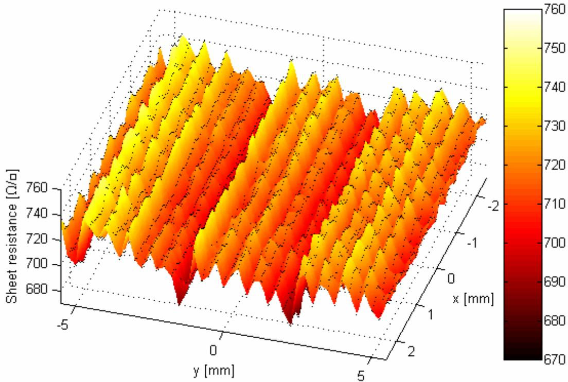
Figure 6: 45x101 point area scan measured with a 10  $\mu\text{m}$  pitch M4PP. The scan step size is 50  $\mu\text{m}$  and 250  $\mu\text{m}$  in the X- and Y-direction respectively. Raw data are represented by dots.
