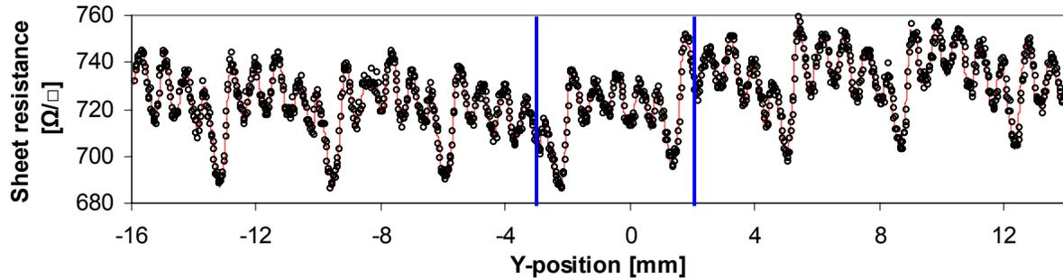
Figure 2: 30 mm sheet resistance line scan perpendicular to the laser scan direction using a 10  $\mu\text{m}$  pitch four-point probe and a step size of 25  $\mu\text{m}$ . The vertical lines define the area which was consecutively probed with different probe pitches (cf. figure 3). A continuous function of the sheet resistance was approximated (thin line) for finite element method (FEM) simulations, cf. figure 9.
