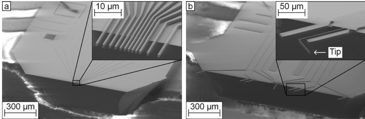
Figure 1: SEM micrographs of (a) a multi-cantilever probe with minimum electrode pitch of  $1.5\text{ }\mu\text{m}$  and (b) a  $500\text{ }\mu\text{m}$  pitch four-point probe with L-shaped static contact cantilevers.
