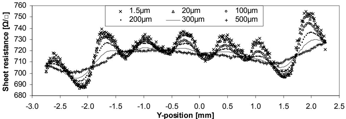
Figure 3: Raw data of a 5 mm line scan with 25  $\mu\text{m}$  step size repeated at the same location with various pitched four-point probes to compare macro and micro sheet resistance. Only selected probe pitch results are shown for easy comparison.
