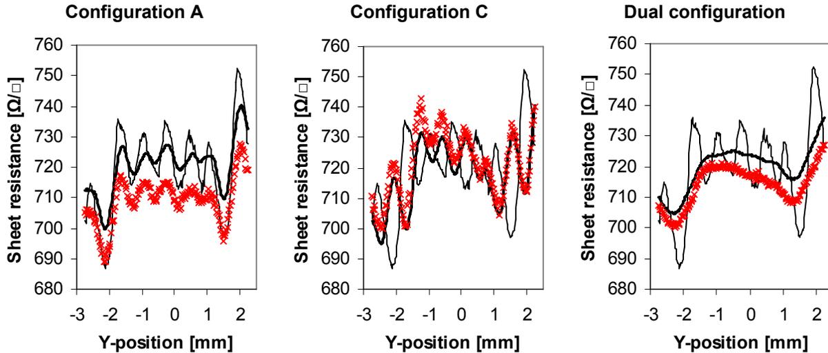
Figure 9: Comparison of configurations A, C and dual for a 500  $\mu\text{m}$  pitch four-point probe on a non-homogeneous USJ. The thin line represents the surface sheet resistance as defined for the FEM simulations (which corresponds to the sheet resistance measured with a 10  $\mu\text{m}$  pitch M4PP). The thick line is the FEM simulated result and the cross represents the experimentally measured result (raw data).
