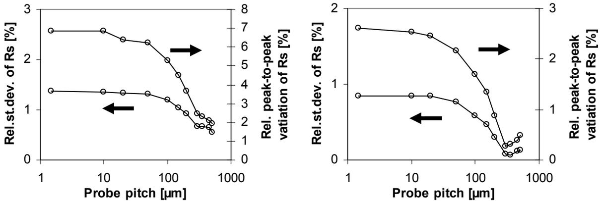
Figure 4: Comparison of the relative standard deviation and relative peak-to-peak variation of the sheet resistance measured with different probe pitches for (left)  $Y = [-1.825 ; 1.825]$  mm (cf. figure 5 left) and (right)  $Y = [0.10 ; 0.85]$  mm (cf. figure 5 right).
