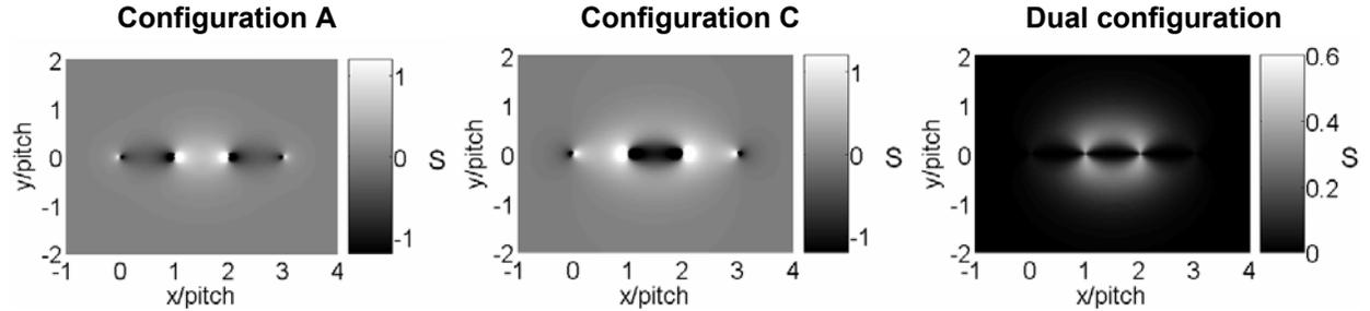
Figure 8: Contour plots of the sensitivity to resistance variations for an in-line four-point probe in the A, C and dual configuration mode. The four contacts are positioned at  $(x,y) = (0,0), (1,0), (2,0)$  and  $(3,0)$ . The sensitivity goes to  $\pm$ infinity at the contact points for the A and C configuration, however the color scale has been cut off (at  $S = \pm 1.2$ ) to see the surrounding contour. The color scale has not been cut off for the dual configuration contour plot.
