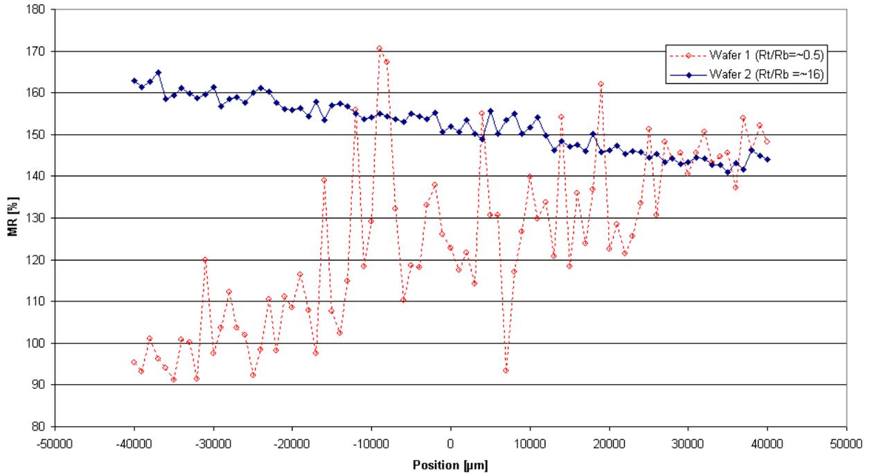
MR vs. position for 2 wedge-wafers; one (Wafer 1) with unsuitable  $R_t/R_b$ -ratio (equal to approx. 0.5), and the other (Wafer 2) with improved  $R_t/R_b$ -ratio (equal to approx. 16). Both wafers had almost similar MTJ-stacks, and similar measurements conditions were used in both cases.
